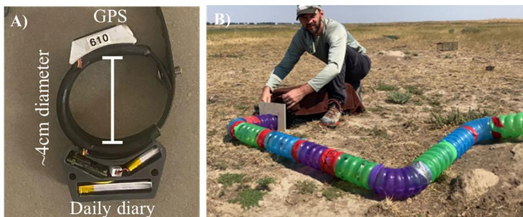
**Fig. 1** Technology and apparatus used to assess dead-reckoning potential for prairie dogs. **A** Photo of the logging system deployed on prairie dogs; **B** with example of constructed tube run with trap connected
