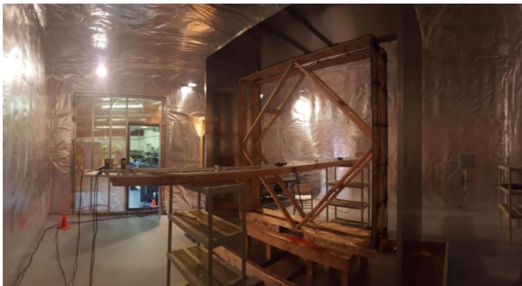
**Fig. 1** Photo of the 1/2-scale model of the BCC antenna. Note the RF shielded room, aluminum shield and pneumatic shuttle (from Axel et al. 16)
