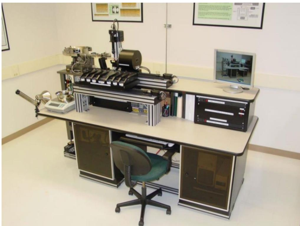
**Fig. 2** Photo of the automated PIT tag testing system (from Axel et al. 16)
