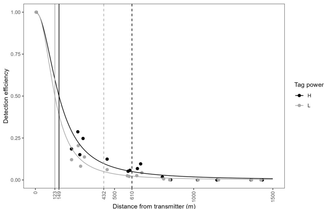
**Fig. 3** Dose–response curves and mean detection efficiencies for high (H) and low (L) power tag transmissions at a range of set distances between tag and receiver pairs. Points represent the hourly detection efficiencies of each pair, averaged over a period of 25 d. Midpoint (50%) and maximum (5%) detection ranges are indicated by the solid lines and dashed lines, respectively
