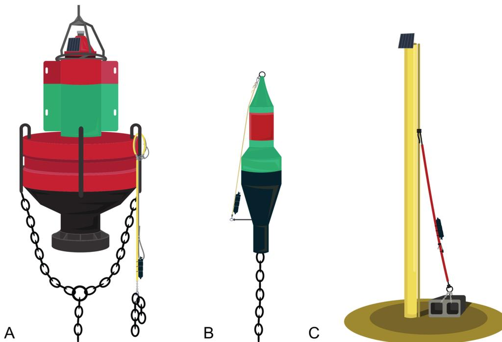
**Fig. 2** Receiver attachment designs for the Swimway array and range test arrays. **A** Large buoy attachment with downward-facing receiver. **B** Small buoy (spar) attachment with downward-facing receiver. **C** Fixed pole attachment with upward-facing receiver and range test tag
