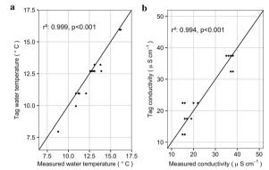
**Fig. 4** Comparison conductivity and temperature measured with the tag and a temperature/conductivity meter. Panel **a** shows water temperature and panel **b** shows the conductivity
