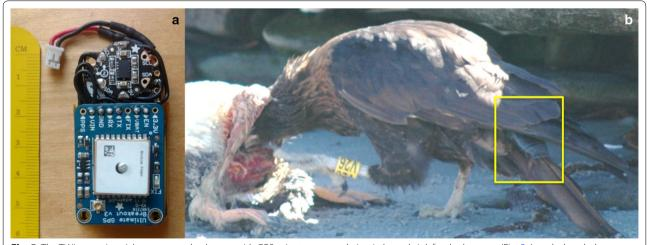
Fig. 5 The TWLogger inertial movement datalogger with GPS prior to encapsulating in heat shrink for deployment (Fig. 5a), and a banded caracara wearing a tail-mounted TWLogger (Fig. 5b) while feeding on a gentoo penguin carcass at the seabird colonies site
