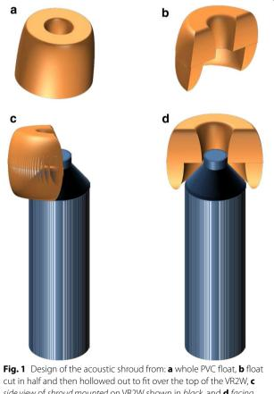
side view of shroud mounted on VR2W shown in black, and **d** facing view
