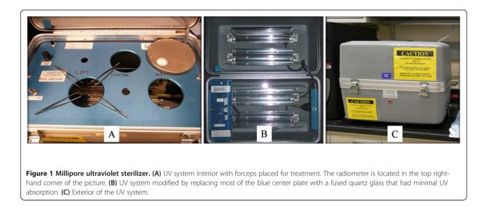
of optical-grade fused quartz glass for UV light at 254 nm is approximately 90% [34].
